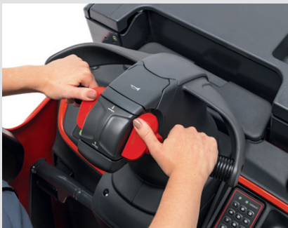
Ergonomic, height adjustable control handle
